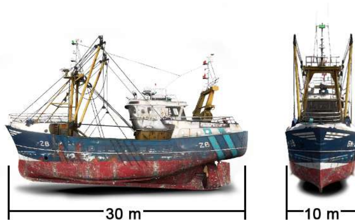
Figure 4.29: Illustration of the dimensions of a typical 1000GT vessel used for the shadowing analysis
