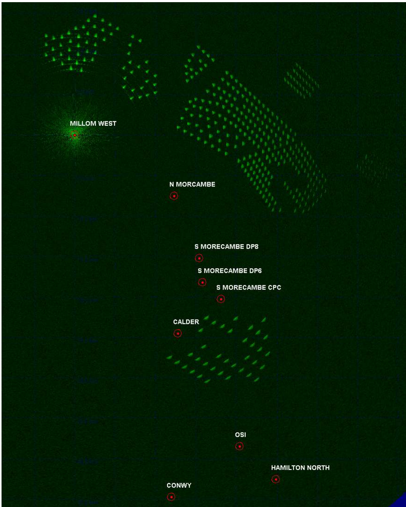
Figure 4.20: Harbour Energy's Millom West platform REWS clutter map showing returns from the Morecambe Generation Assets wind turbines and sea clutter.
